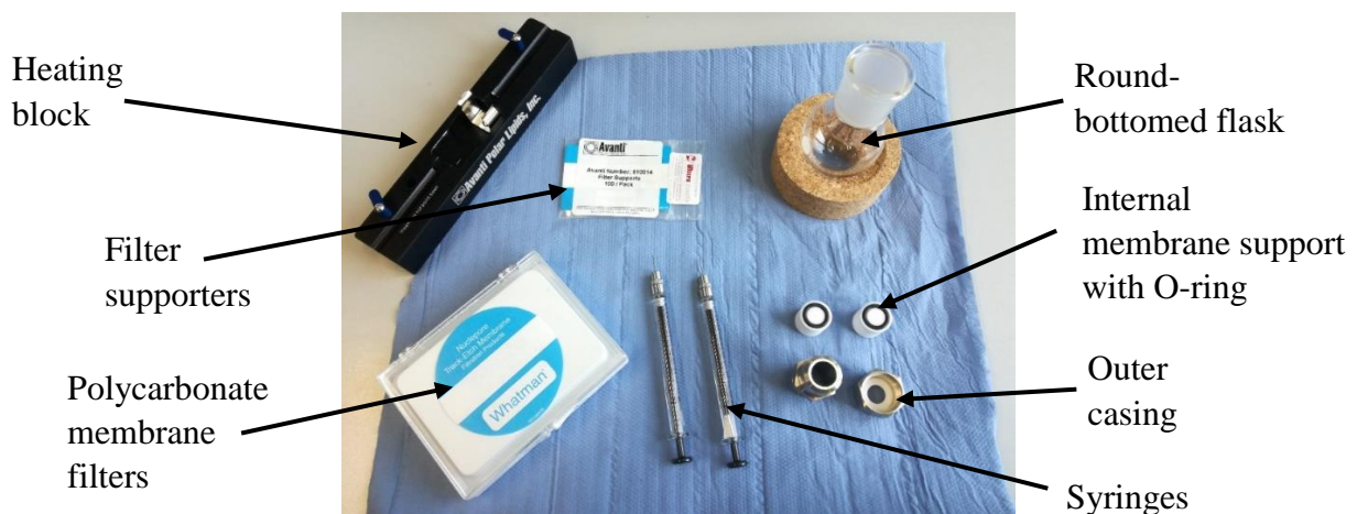
Figure 17: Setup for the extrusion process. Heating block, round-bottomed flask, syringes, polycarbonate membrane filters, filter supporters, teflon holders and outer casing to hold it all together
