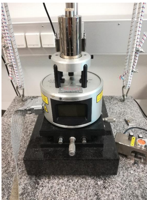
Figure 24: Multimode AFM used for the experiments
