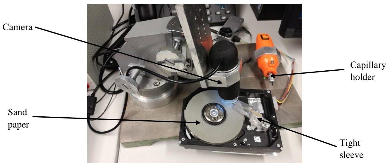
Figure 14: Setup for capillary tip sharpening
