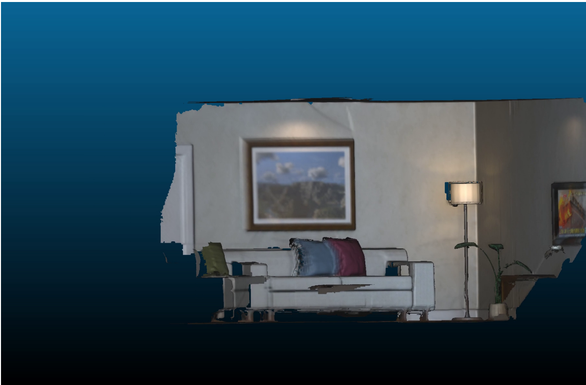
Figure A.2: Impact of the principal point error on the reconstruction.
