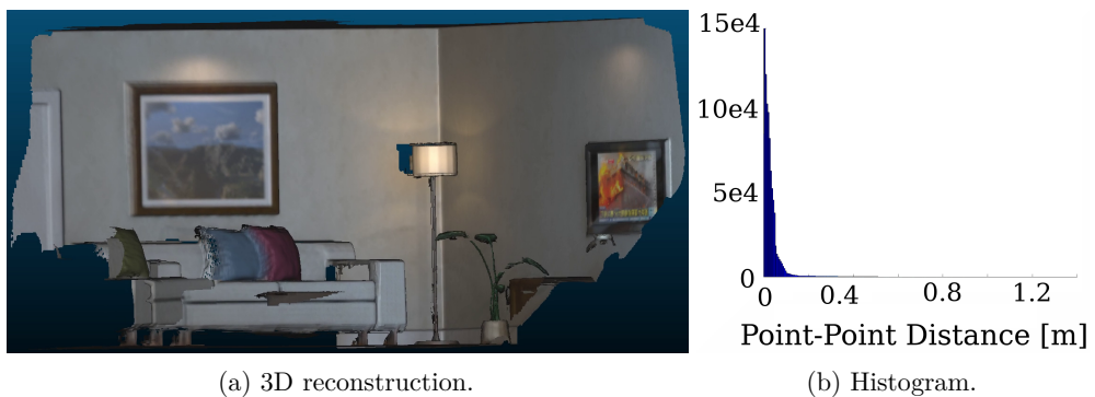
Figure 3.8: Reconstruction generated with perfect depth and camera pose information. The generated 3D scene and the error histogram of the cloud-cloud distance between the CAD data and the reconstructed scene represent the baseline, and the absolute limits of the used reconstruction algorithm.
