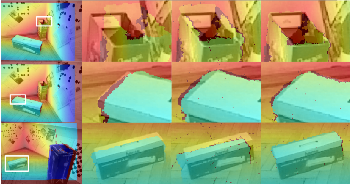
Figure 5.6: Qualitative results of the calibration. From left to right: scene, initial parameterization, reference method (IPD, [32]), the introduced method that gives the best qualitative result, using PLD, IPD, and WIPD. Figure best viewed in color.
