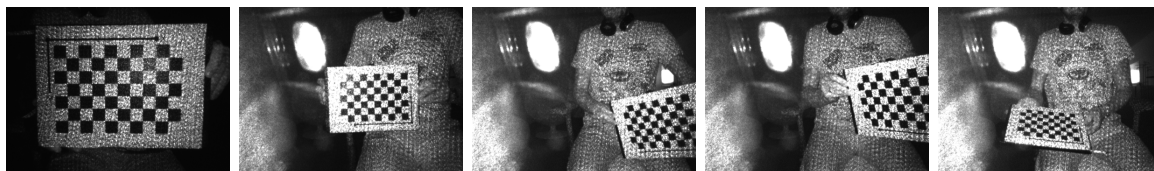
Figure 5.1: Camera Calibration to get the intrinsic parameters of the used R200 Active Stereo camera.
