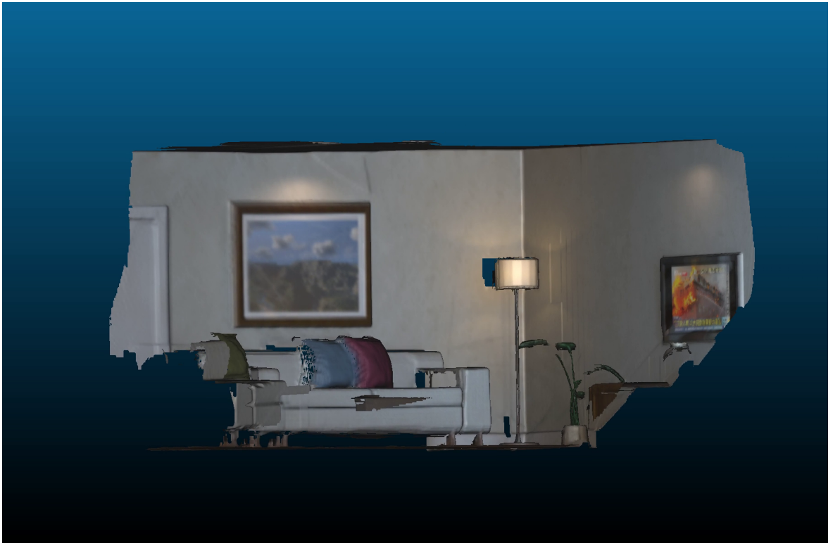
Figure A.3: Impact of the focal length error on the reconstruction.
