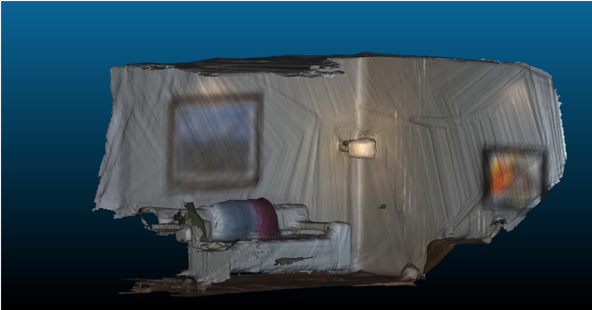
Figure A.9: Impact of the camera pose error on the reconstruction.
