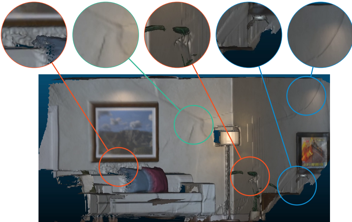
Figure 3.9: Impact of the interpolation error (orange), radial distortion error (blue), and tangential distortion error (turquoise) on the image quality.
