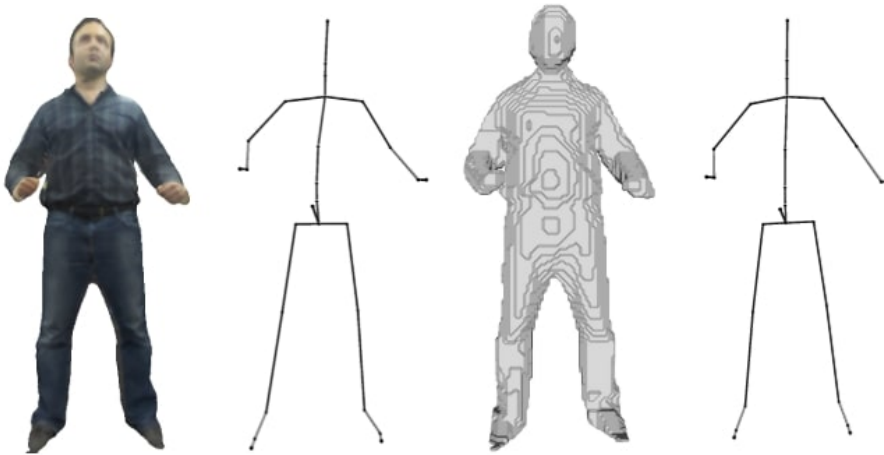
Figure 3.8: On the left the original mesh of the human 3D scan and the corresponding skeleton. On the right the voxel representation of the mesh using the depth buffers and the skeleton of it. It can be seen that the skeletal representation looks the same for both representations of the 3D model [SFW + 14].
