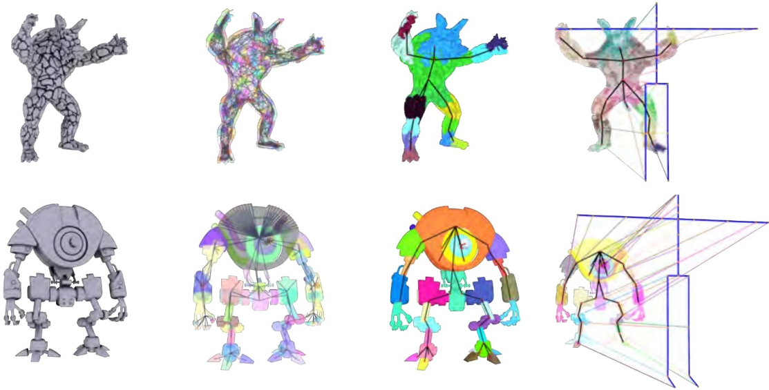
Figure 3.9: Two multi component models rigged by the approach of Bharaj et al. [BTST12].
