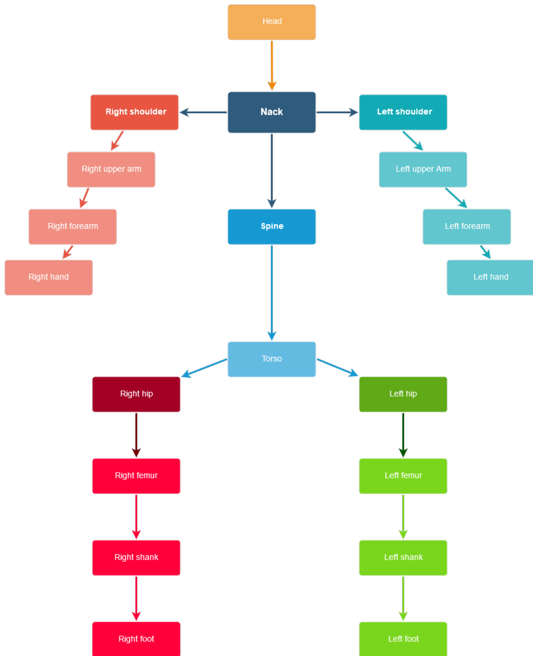
Figure 4.9: Schematical representation of the armature used in bender consisting of 20 segments and 18 joints.
