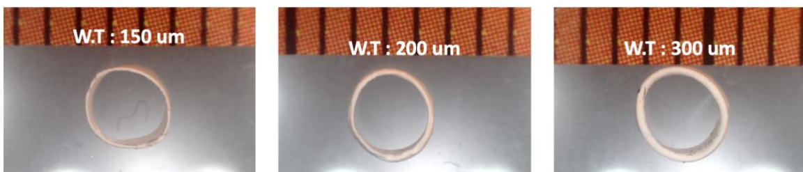
Figure 2.4: Varying electrospun time and the resulting wall thickness.
