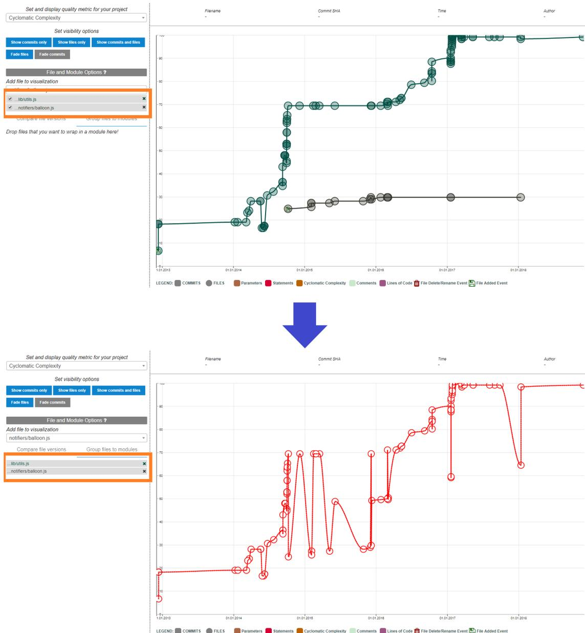
**Figure 5.9:** The screenshot above shows two files that are selected and displayed in the file list. Moving the files to the group panel via drag and drop in the screenshot below computes the average of the quality values, *Cyclomatic Complexity* in this case, of the two files. Note that the computation of average values only applies to commits that have modified both files.
