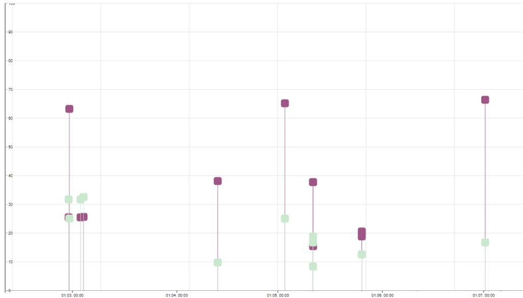
**Figure 5.5:** Example state of the trend chart area with commits. Two quality metrics for commits are displayed to be able to compare them to each other. The metric *Lines of Code* is magenta and the metric *Comment Lines* is light green. One possible interpretation of the chart could be that the ratio of *Comment Lines* to *Lines of Code* has decreased over time.
