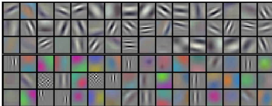
Figure 3.3: The 96 learned filters of size 11 \times 11 \times 3 from the first convolutional layer of AlexNet [14] on the 224 \times 224 \times 3 input images. Each filter represents a special pattern that steers the distillation process in the convolutional layer. The network has learned a variety of frequency- and orientation-selective filters and different coloured blobs.
