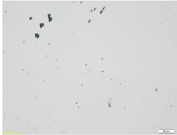
Abbildung 13: LOM: Al HEA-Ingots, V2A-Beize 30s
