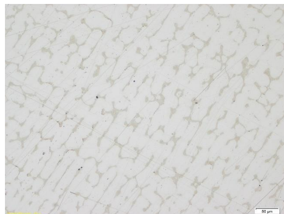
Abbildung 55: LOM: A4 HEA-Ingot, V2A - Beize 30s
