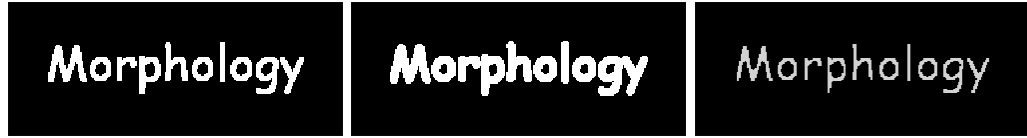
(a) Original image A . (b) Dilated image A \oplus S_8 . (c) Eroded image A \ominus S_8 .
