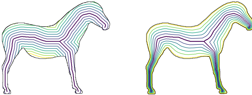
(a) Distance coordinate r on a horse shape. Purple contour at 0, yellow at 70. (b) Scaled coordinate r_s on a horse shape. Purple contour at 0, yellow at 1
