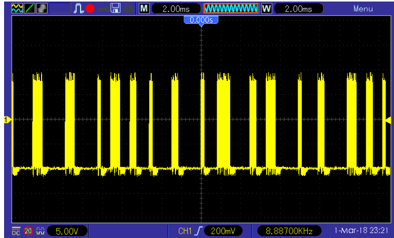
Figure 6.3: Test of transmitter module: The oscillogram shows the carrier frequency which is modulated (turned on and off) by a modified gold code sequence.
