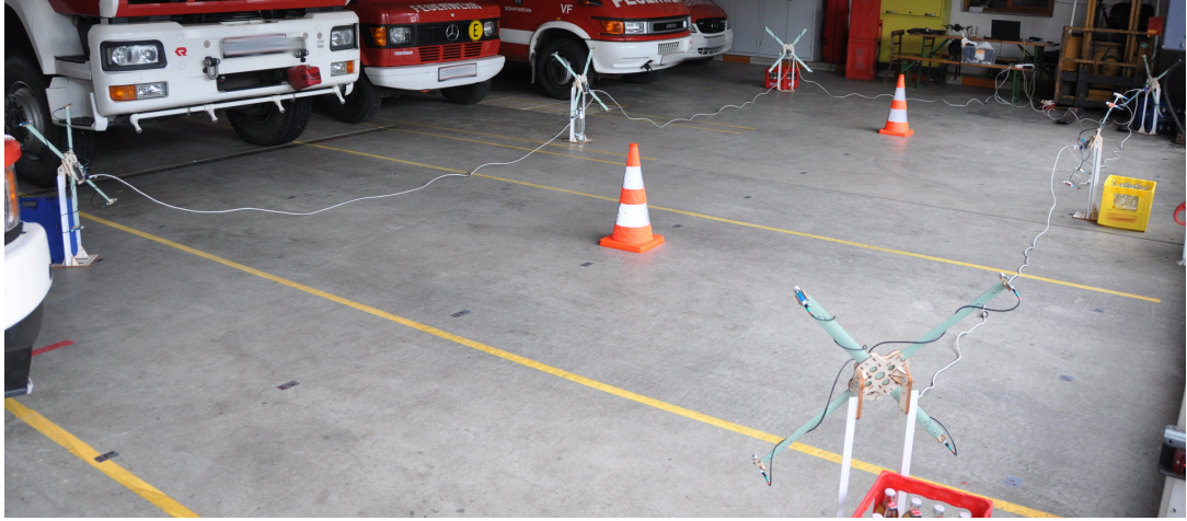
Figure 6.19: Autopilot test area setup with a dimension of x_{max} = 10m and y_{max} = 5m . The four of the base stations are placed on the corners of the test area and two on the border at x = 5m . The centers of the 8-figure (reference flightpath) is marked by orange traffic cones.
