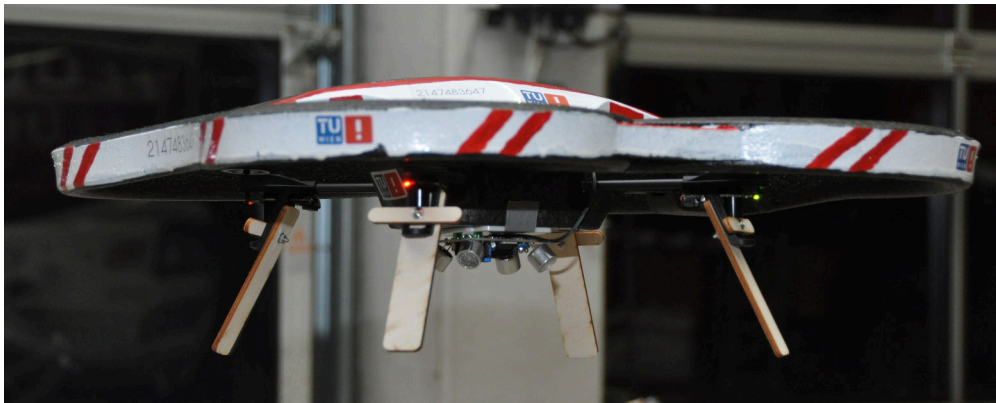
(b) Bottom side of the UAV which is used for the dynamic tests. The transmitter module v2.2 is placed in the center on the bottom of the UAV.
