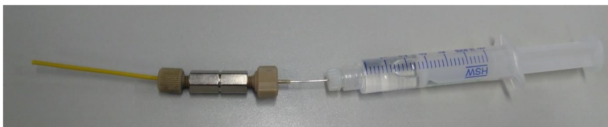
FIGURE 26: SYRINGE ADAPTER TO FIT CAPILLARY TIGHTLY
