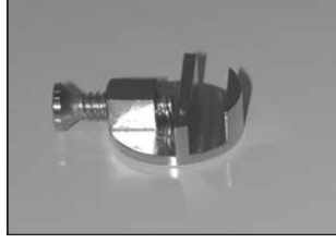
Figure 3.9: Cross sectional sample holder for SCM applications. The screw is used to fix the sample and to establish a good electrical contact.
