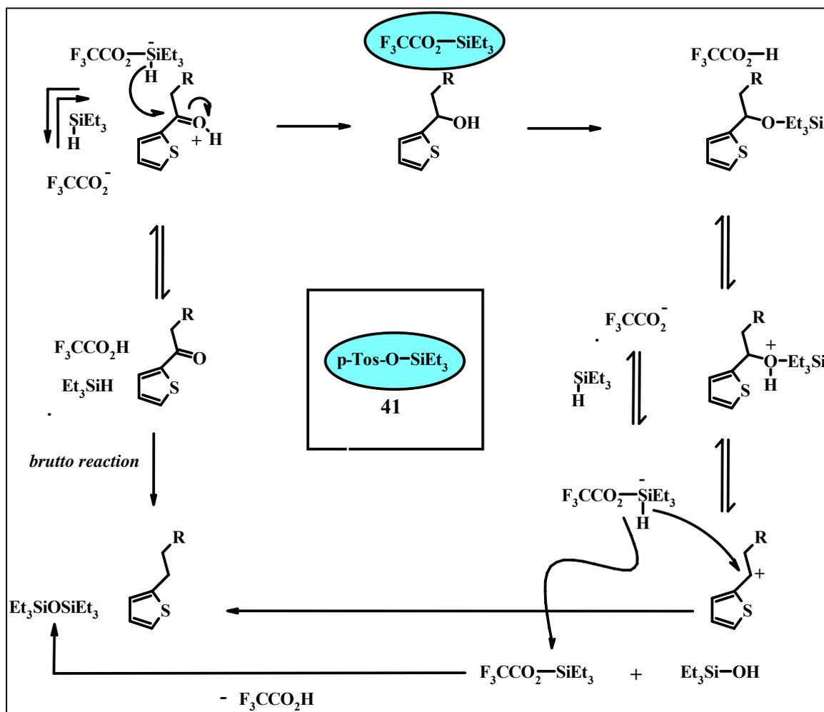
Scheme 52: Mechanism of the acidic deoxygenation
