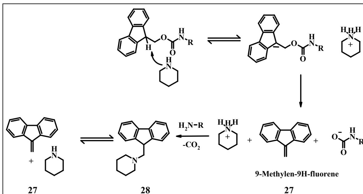
**Scheme 44: Mechanism of the cleavage of the Fmoc-group**
