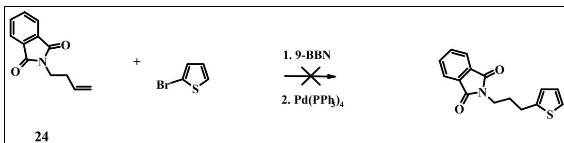
**Scheme 41: Test reaction for Suzuki-Coupling approaches**
