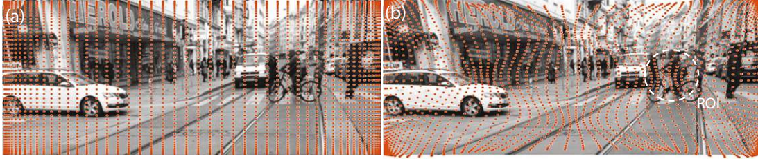
Figure 7.13.: Conceptual illustration of conventional Lissajous scanning (a) and ROI scanning using the proposed method (b) in a lidar scenario. Significantly more measurement points are created in the ROI compared to the conventional method.
