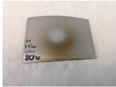
Figure 4.9: Image of sputtering test 2 on a silicon wafer, distance of 5 cm, plasma power of 80 W
