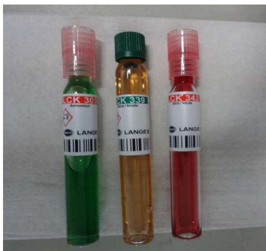
Figure 13. Standard cuvette tests used to detect spectrophotometrically the amount of ammonium (green cuvette), nitrates (yellow-orange cuvette) and nitrites (red cuvette).
