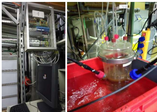
Figure 11. The 3 L bioreactor immersed in a heated water bath (right) and the control PC (left).
