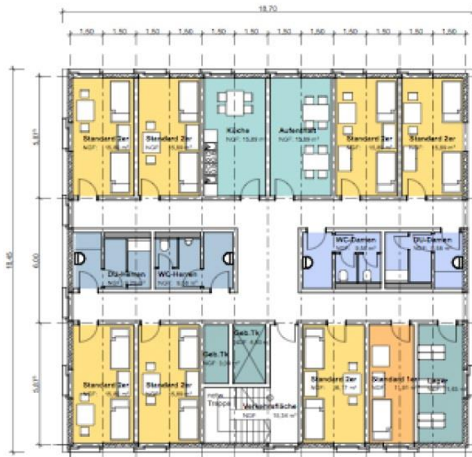
Figure 27 Upper floors of MUF's module: 7 standard rooms of 16 m 2 and 1 standard room of 11 m 2
