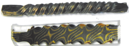
Figure 1: Twisted bar; overall view and longitudinal section with torsion pattern.
