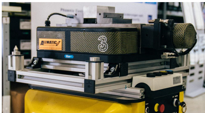
Fig. 3. Smart clamping pallet placed on an AGV.
