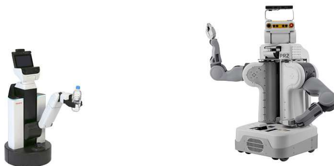
Figure 5 Two domestic service robots. Left: Toyota Human Support Robot (HSR). Right: PR2 by WillowGarage.
