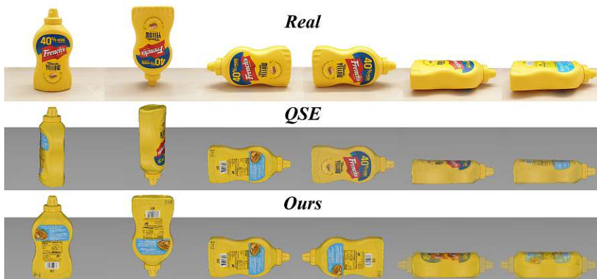
Figure 6 Stable object poses. Top to bottom: The real object, QSE [Goldberg et al. 1999] and our approach for isolated objects (ours). Multiple representatives of the same stable pose are transparently overlaid for QSE and ours. Reprinted from [Bauer et al. 2020a].
