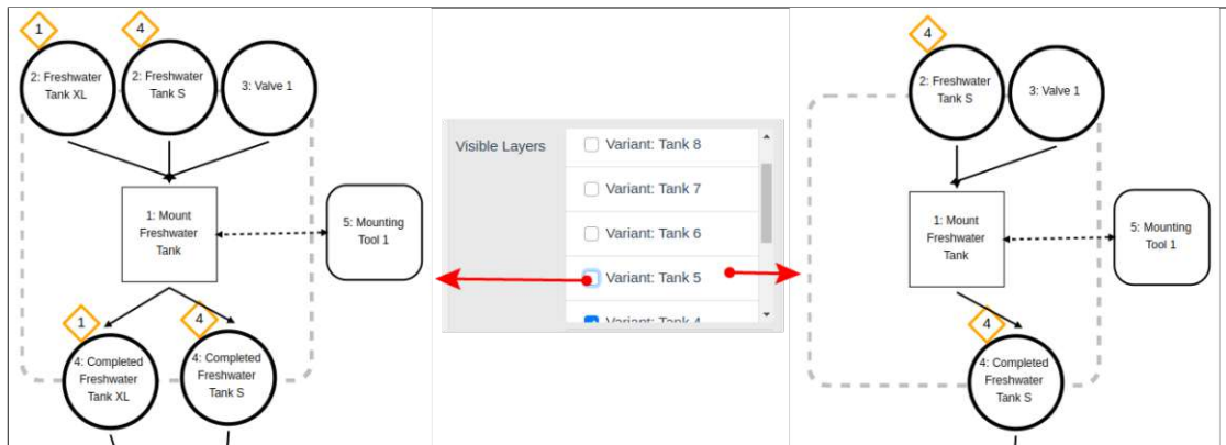
Figure 7.14: TC-2.6 - Hide Features of Superimposed PPR Model using the Layer Toggle of the VME Modeling Component
