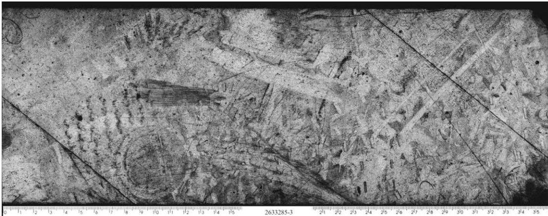
Figure 4.11: Real crime scene footwear impression(s) collected using a gelatin foil lifter.
