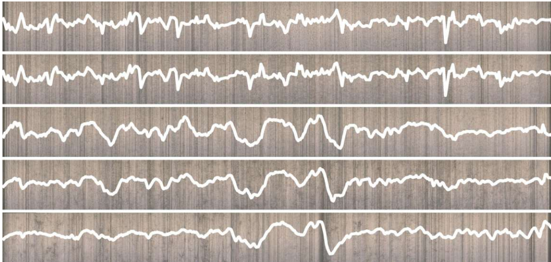
Figure 4.2: Superimposed 1D profiles extracted from 3D surface scans onto 2D images of the NFI Toolmarks dataset [BKP + 14]. All marks were made by the same tool with varying angle of attack; from top to bottom: 15 degree, 30 degree, 45 degree, 60 degree, and 70 degree.
