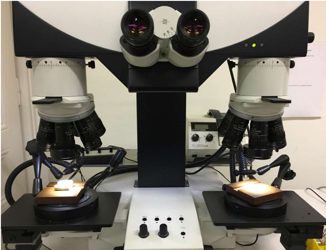
Figure 3.3: Leica comparison microscope which was used for capturing the toolmark images.
