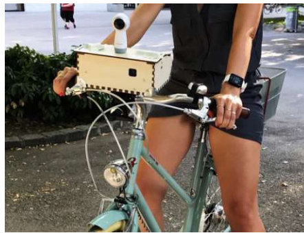
Figure 6.4: Hardware iteration of the Virtual Cycling Coach used in the second evaluation round: Mounted on the handlebar, the casing housed a front-facing camera that live-streamed a video feed to the controlling researcher (the wizard), a smartphone with an attached speaker for outputs of the audio interface, and a 360° camera on top for recording the session.
