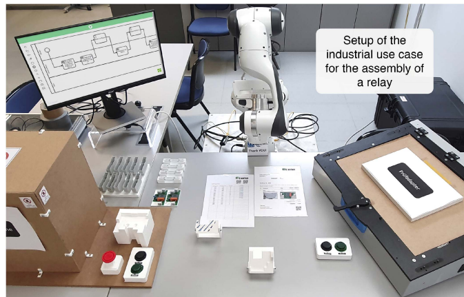
Fig. 1. Cobot demonstrator including user interface for adaptive task sharing and industrial use case.
