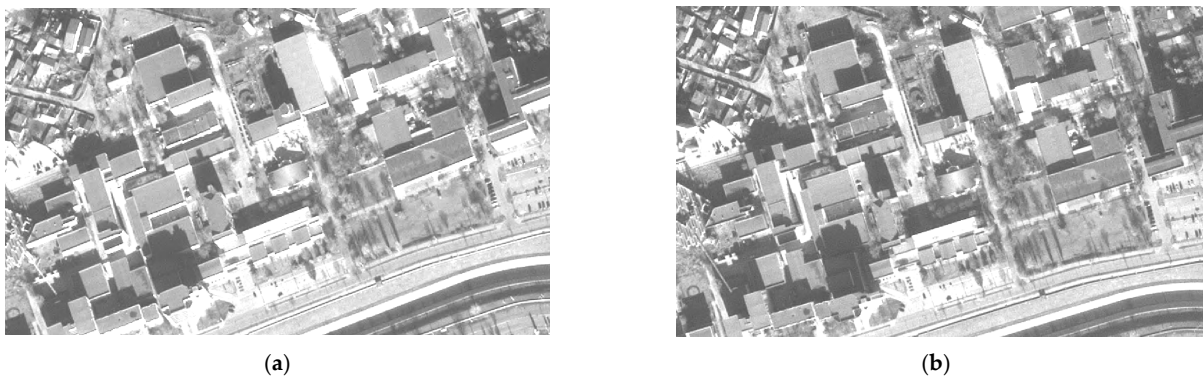
Figure 5. Detail of Pléiades satellite images in panchromatic band on the same area: (a) forward-looking image, (b) backward-looking image.
