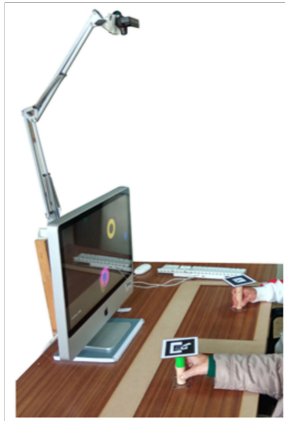
Figure 2.7: Game Setup: Camera and Handles with Tracking Pattern [77]
