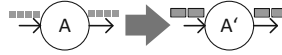
Figure 2.14: Communication and processing of data can be adapted to use larger batches of events instead of handling them independently [HSS + 13].
