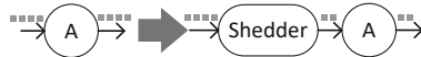
Figure 2.10: Example of discarding events when the processing capacity is exceeded to ensure maximum throughput and stability for the application [HSS + 13].
