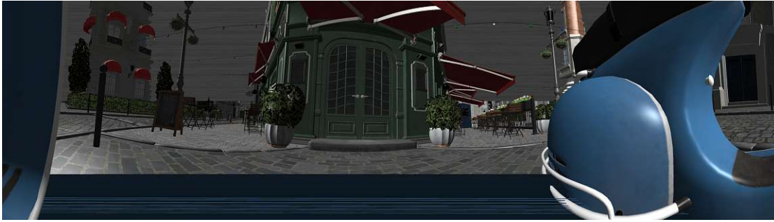
Figure 4.5: Severe rasterization artifacts in a 360° rendering where triangles spanning the discontinuity at \pm\pi are rasterized over the entire width of the screen.
