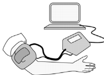
Figure 49: non-invasive device for measurement of central aortic pressure changes [Gorenberg et al., 2005]
