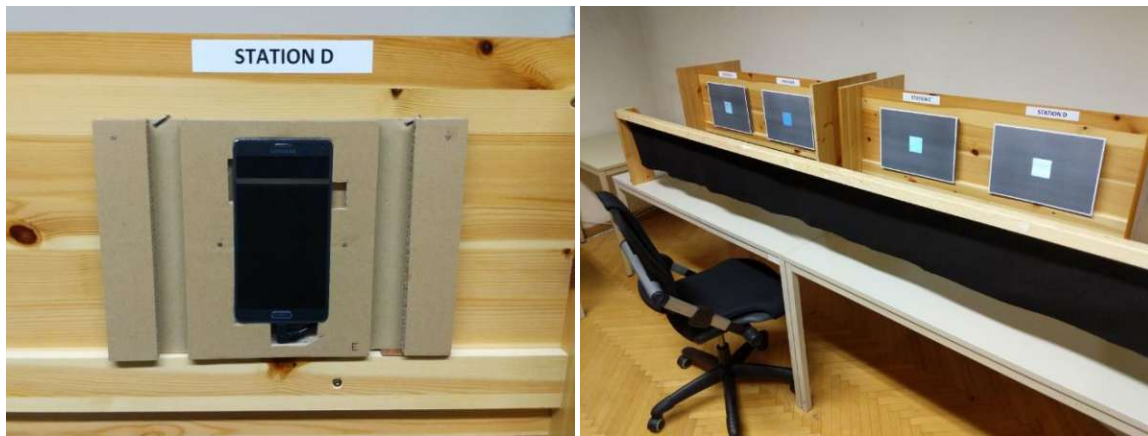
Figure 4.2 Left: adapter module to accommodate a mobile phone for the study, made from corrugated cardboard. Right: The two shelves constructed for the experiment, each holding two adapter modules, with grey bezels revealing only a portion of the screen of each device. A chin rail with a curtain to prevent reflections is mounted in front of the shelves.
