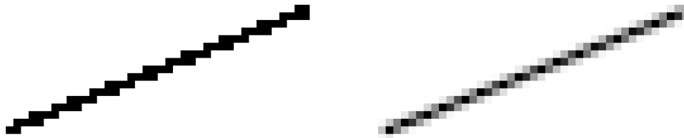
Figure 3.12 Aliasing and antialiasing. Left: rendering a line at an oblique angle as a bitmap image results in a jagged appearance (aliasing). Right: Antialiasing substitutes spatial resolution with intensity resolution, colouring partially-covered pixels in shades of grey, which results in a smoother appearance at equal display resolution.
