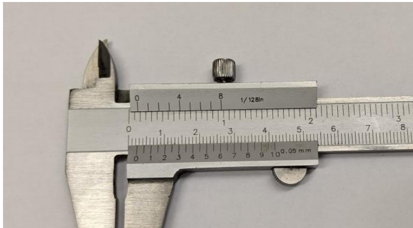
Figure 3.5 Vernier scale on a calliper. Because the human eye is very good at detecting the alignment of collinear lines, the line in the lower part that lines up precisely with one of the lines on the millimetre scale can be easily identified (the line numbered “6” at the bottom), and conveys the fractional component of the measured distance (in this case: 2.6 mm).
