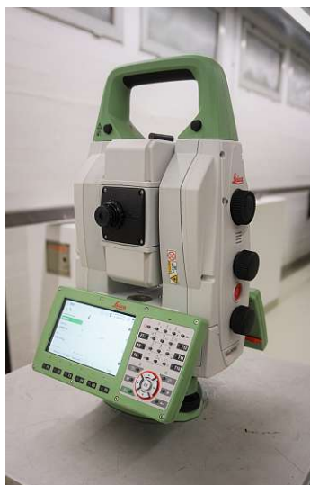
Figure 2.2 & Table 2.2: Accuracy specifications ( 1\sigma -values) and technical characteristics of the used multi station Leica MS60 stated by the manufacturer (Leica Geosystems 2020).
