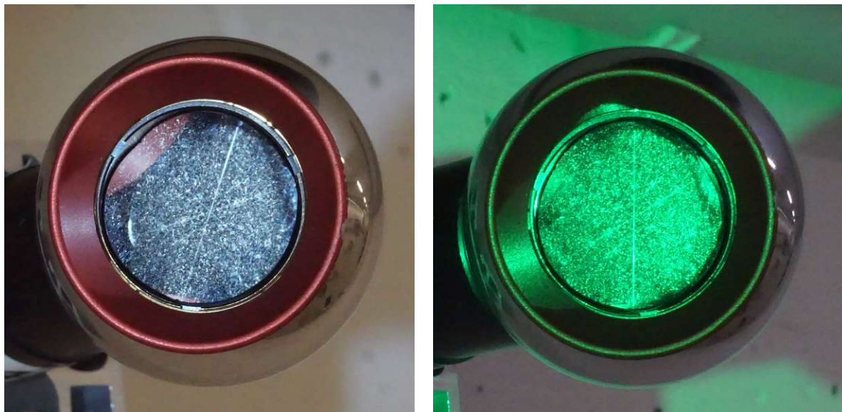
Figure 5.6.: Illumination of the corner cube reflector by white and green light. The visual impurities on the cube surfaces are caused by dust particles.
