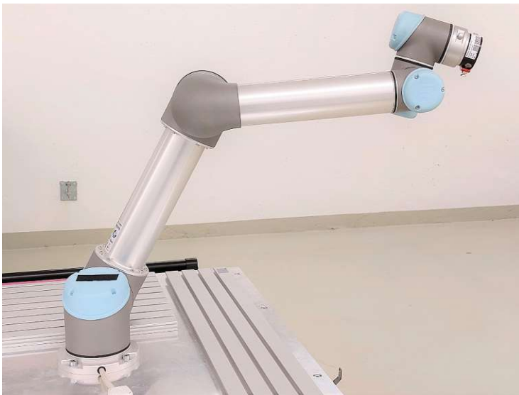
Figure 2.6 & Table 2.6: Specifications of robot arm UR5 (Universal Robots 2016)
