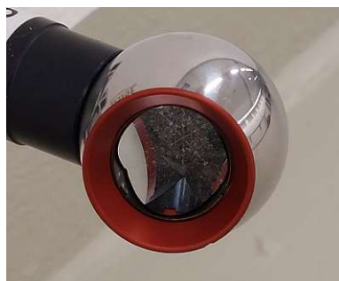
Figure 2.5 & Table 2.5: Specifications of Leica Red Ring Reflector 1.5'' (Hexagon Metrology 2022).
