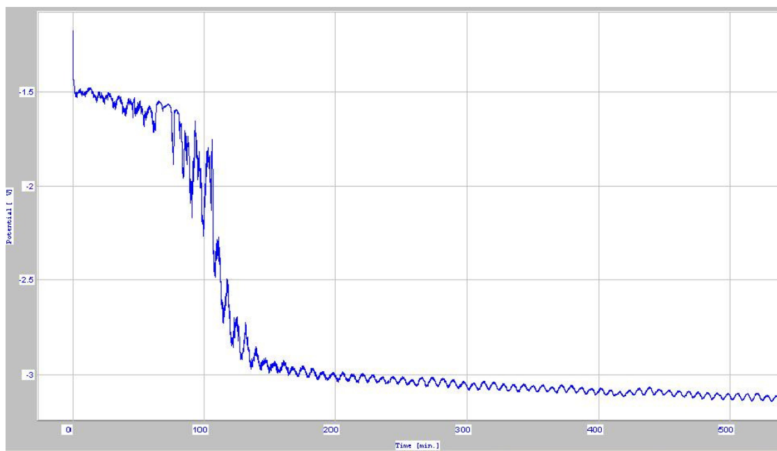
Fig. 3.62 Change of the potential between the cathode and anode during electrolysis.
