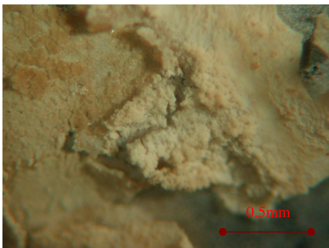
Fig. 3.63 Obtained deposit on a Pt wire (light microscope picture).
