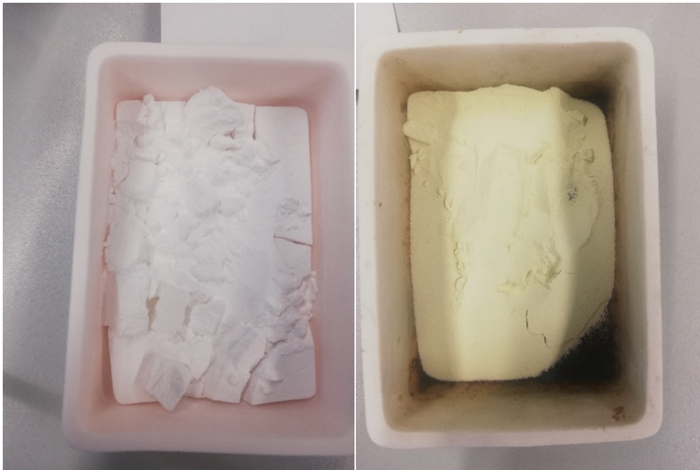
Figure 18: left: Al 2 O 3 "Sasol PURALOX SBA200" after heat treatment (1150 °C) without change of color; right: Al 2 O 3 "90 active" after heat treatment (1150 °C) with clearly visible yellow coloring
