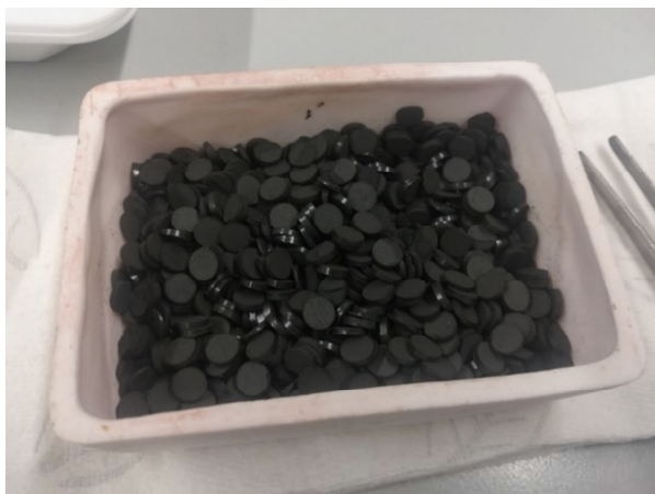
Figure 51: tableted material after calcination
