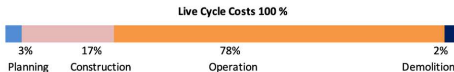
Figure 25: Life cycle costs of a building (Wehrberger, 2022)
