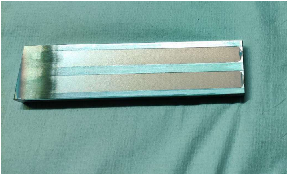
Figure 13: Grind Gauge coated with a thin layer of slurry.
