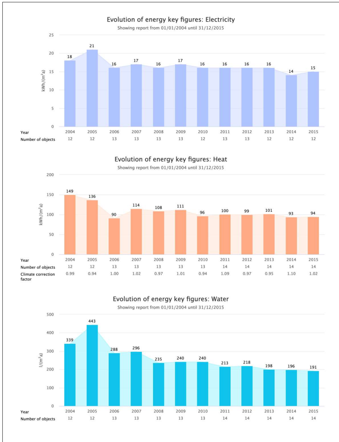
Figure A.3: Key Figure Reports (Electricity, Heat and Water) of a sample community.
