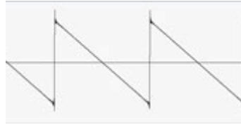
Figure 3: A saw tooth wave, a combination of a sine wave of a certain frequency summed with all harmonics of that frequency. Retrieved from [Preve, 2007]
