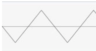
Figure 5: Like the square wave, the triangle wave is the sum of all odd harmonics with their fundamental frequency. Instead of reducing the volume in a linear fashion, the volume is reduced exponentially. Retrieved from [Preve, 2007]
