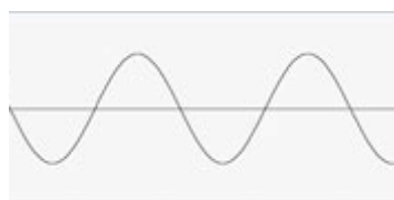
Figure 2: A sine wave, the most basic sound wave. Retrieved from [Preve, 2007]
