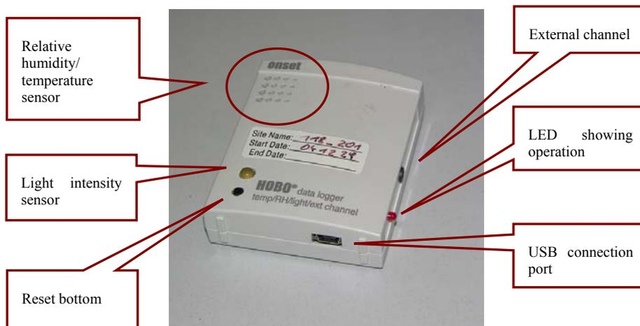
Figure 2-7 Hobo sensor/logger
