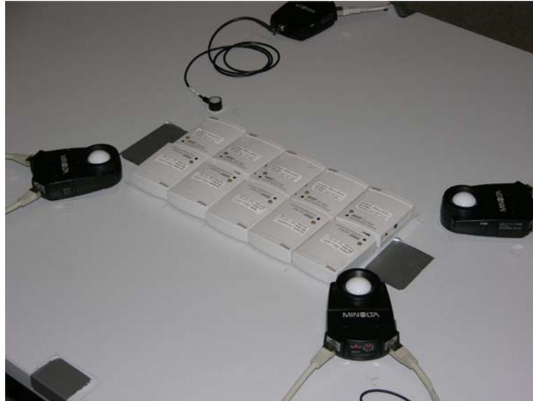
Figure 2-18 process to find the accuracy factor of the light sensors
