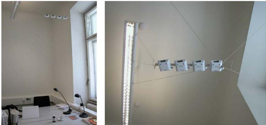
Figure 2-27 Experiments of accuracy of occupancy loggers
