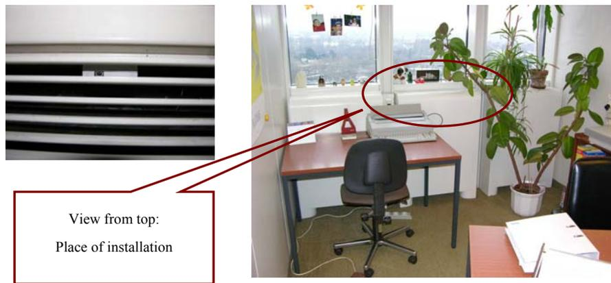
*Figure 2-9 Installation place for temperature logger inside the radiator boxes*
