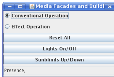
Figure 6.3: Demonstration application for the demonstration suitcase. The checkboxes at the top of the GUI can be used for switching between the operational modes. The buttons below allow to directly affect the building automation system. In the text label at the bottom information delivered by ARS-PC is shown.
