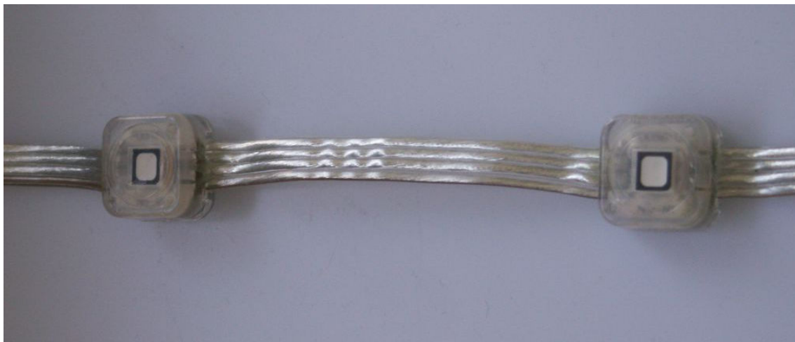
Figure 6.7: LEDs used in the demonstration suitcase to represent a media façade. The LED elements are multi-color. This type of LED string is used in real world media façades.
