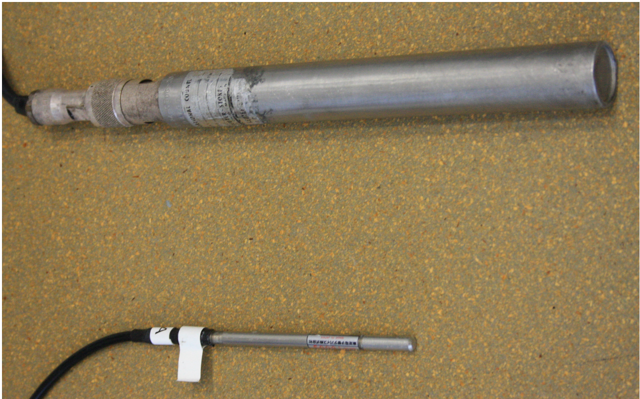
Figure 3.18: Two differently sized He neutron detectors. Both of them were used during the calibration of the final setup for our noise-disturbance measurements.
