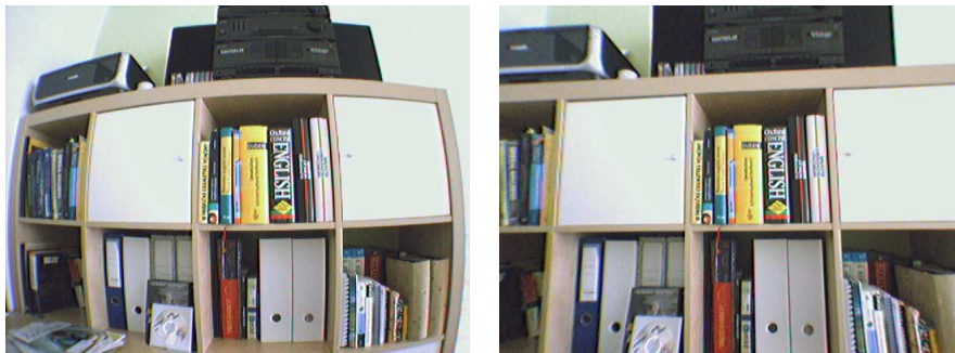
Figure 2.12: On the left side a distorted image taken with a wide-angle lens (2.1mm - horizontal angle is 81^\circ ) is displayed. On the right side an undistorted image is presented.
