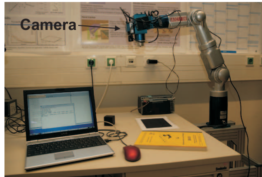
Figure 4.15: The setup for the controlled experiments consists of the gigabit ethernet camera mounted onto a 7DOF robotic arm.
