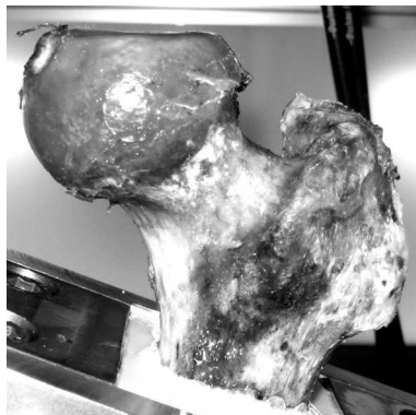
Figure 2.4: Non-clinical-relevant fracture, which was produced in a compression test without embedding the femoral head.
