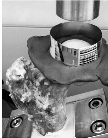
Figure 2.9: Preparing the mold for embedding the femoral head: Before starting the embedding, the loading platen will be lowered to a distance of 10 mm to the femoral head.
