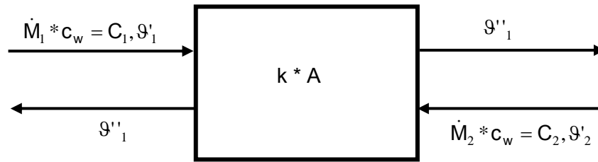
Figure 6-2: Schematic illustration of heat transfer in heat exchangers (own diagram)
