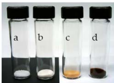
Image 2-1. Photos of (a) \text{MeReO}_3 , (b) silica-alumina, (c) \text{MeReO}_3 grafted onto uncalcined silica-alumina and (d) \text{MeReO}_3 grafted onto calcined silica-alumina.
