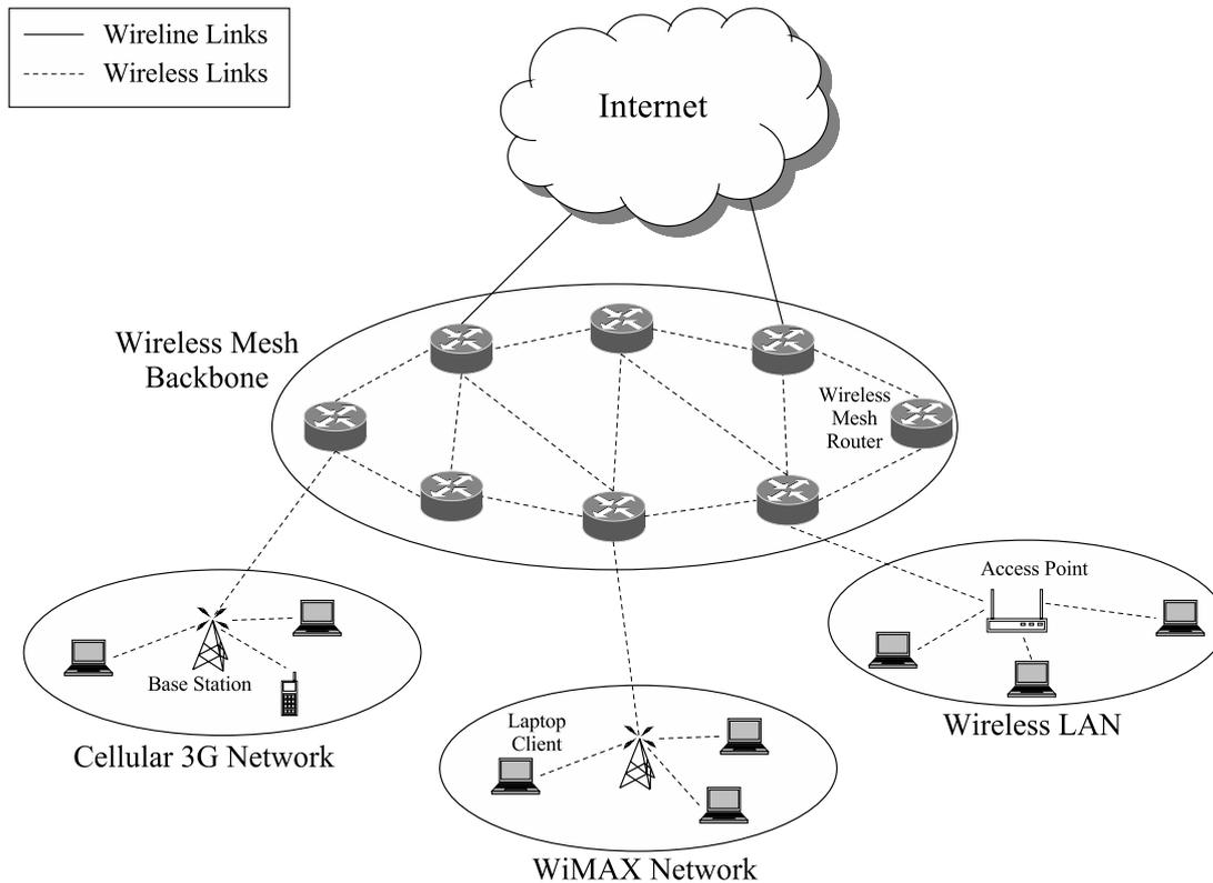
Figure 6.3.1: Example of an infrastructure/backbone wireless mesh network.
