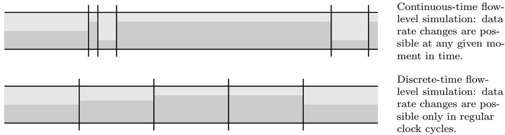
Figure 4.1.2: Difference between continuous-time and discrete-time flow-level simulation.
