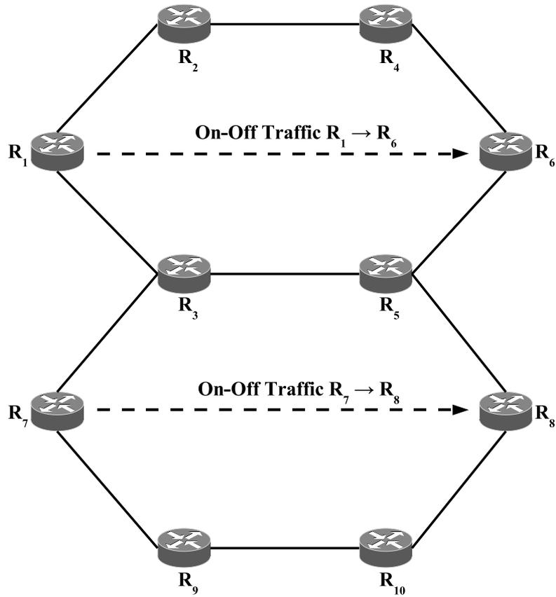
Figure 4.4.6: Setup of Stability Experiment 3 featuring two interfering on-off traffic streams.
