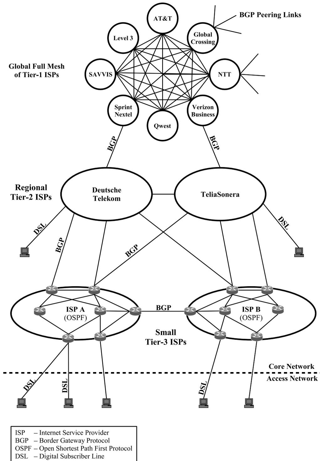
Figure 2.1.1: Current high-level architecture of the Internet.
