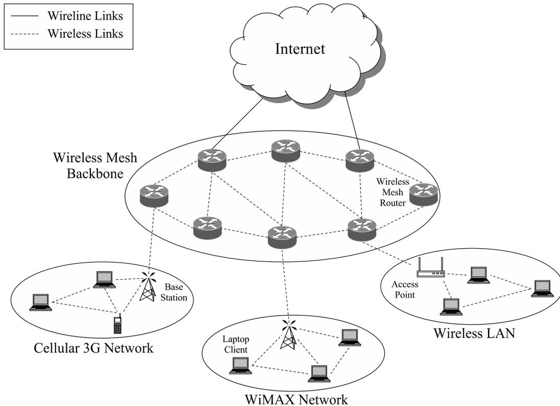
Figure 6.3.3: Example of a hybrid wireless mesh network.
