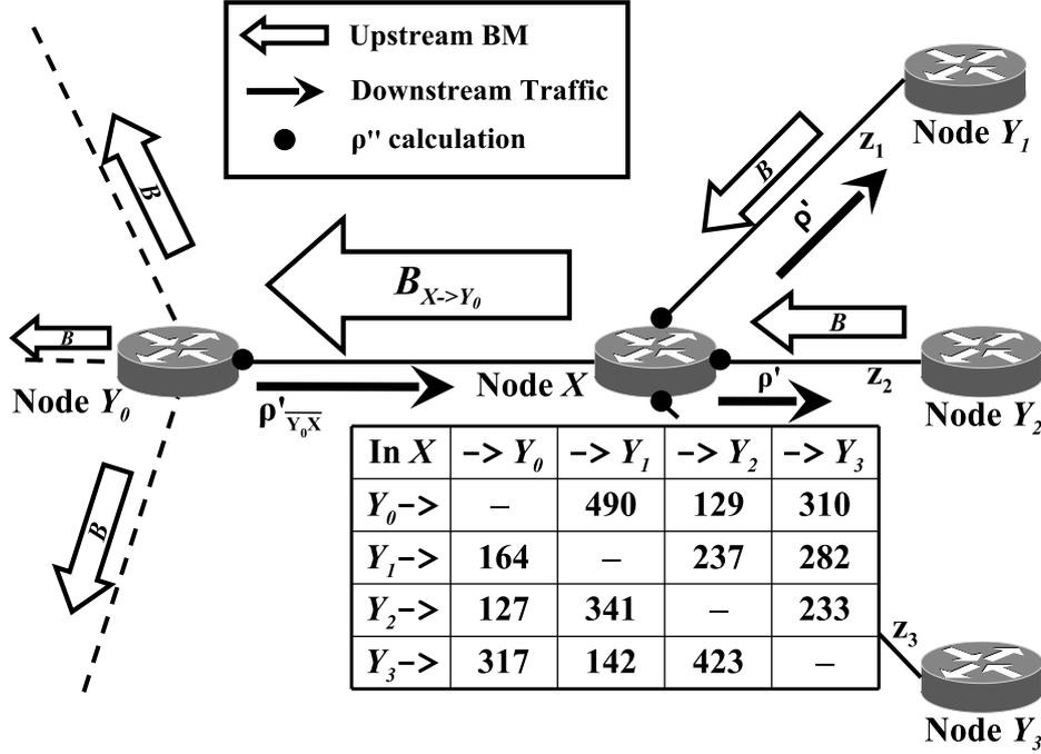
Figure 3.2.4: Example for a Backpressure Message (BM) from  $X$  to  $Y_0$  and *in/out matrix* in node  $X$ .
