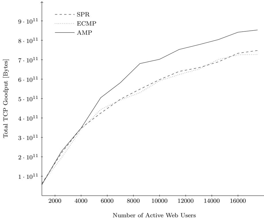
Figure 5.3.2: Total TCP goodput in the AT&T-US network.
