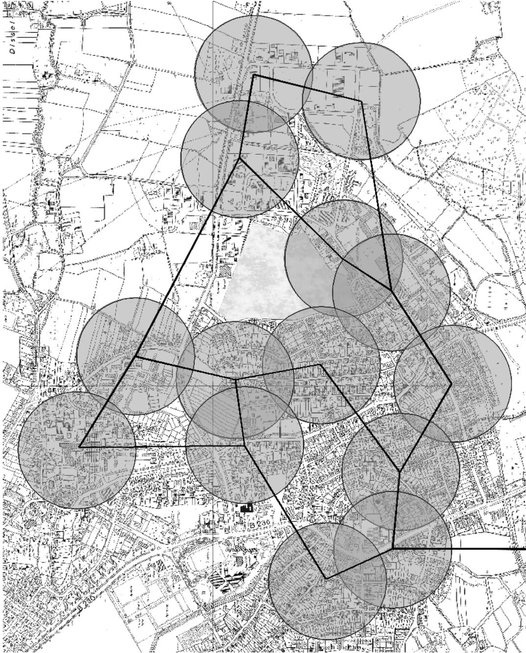
Figure 6.3.4: Local-Web wireless backbone network. (Source: [123])
