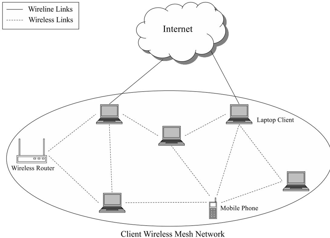
Figure 6.3.2: Example of a client wireless mesh network.
