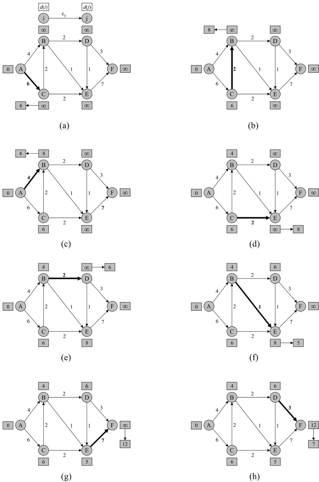
Figure 2.1.4: Illustration of the *generic label correcting algorithm*.
