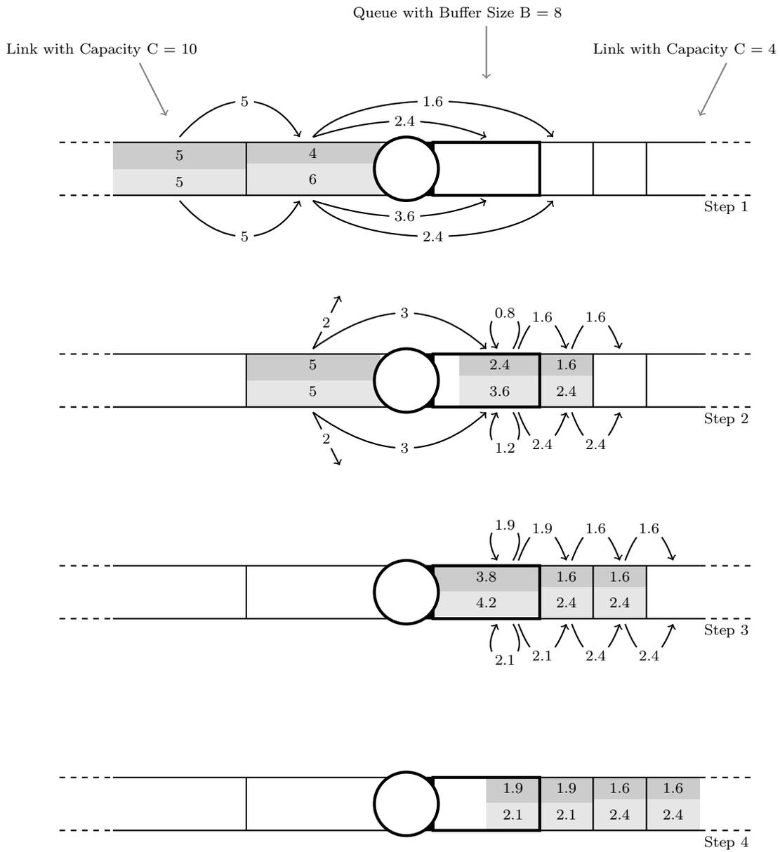
Figure 4.1.3: Example queuing behavior in time-discrete flow-level simulation.
