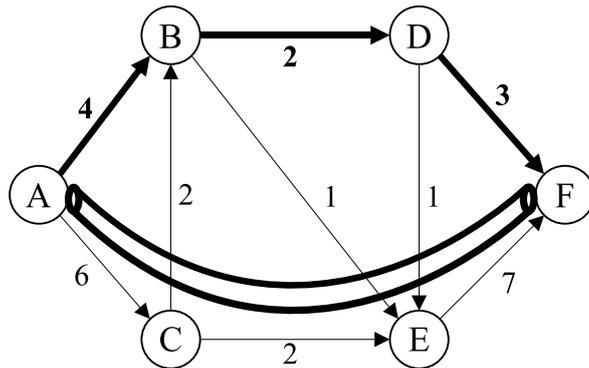
Figure 2.2.3: Arbitrary MPLS tunnel from node  $A$  to node  $F$ ,  $A \rightarrow C \rightarrow E \rightarrow F$  which disregards the shortest path according to the link weights,  $A \rightarrow B \rightarrow D \rightarrow F$ .
