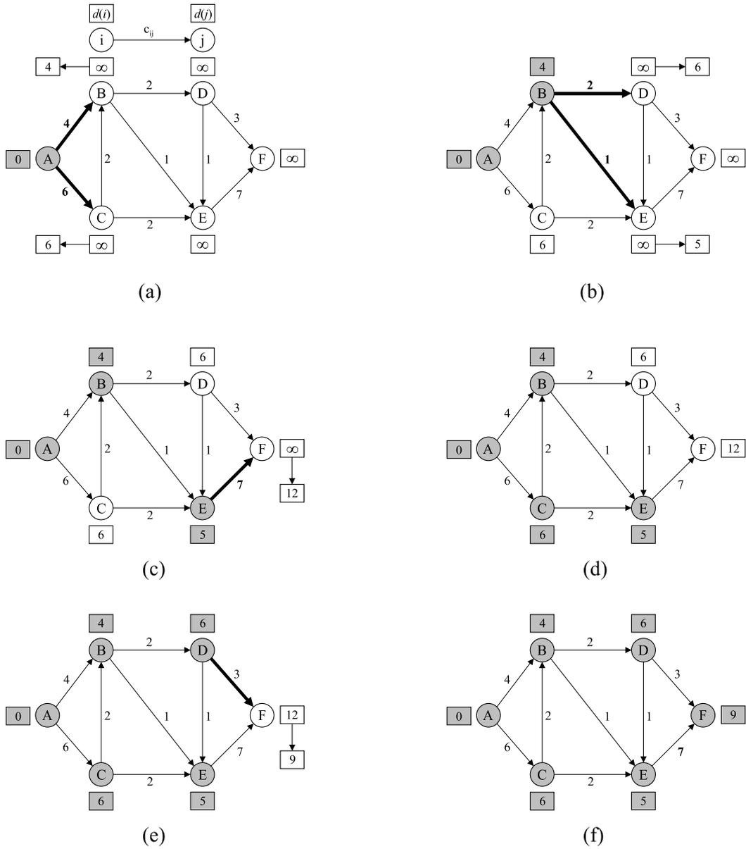
Figure 2.1.3: Illustration of Dijkstra's algorithm (extending Figure 4.7 from [19]).
