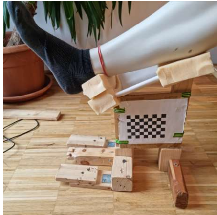
Figure 4.2: Picture of the footrest with a mannequin foot.
