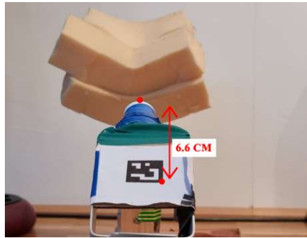
Figure 4.7: Fixed distance between the fiducial marker and the robot for the back camera.
