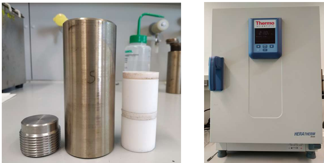
Figure 10: A steel autoclave (left) and an oven (right) used for hydrothermal synthesis.
