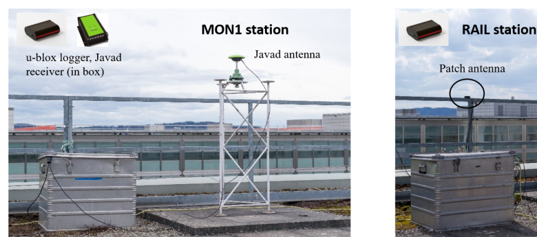
Figure 1. Session 1: experimental setup for station “MON1” for the static kinematic tests (left-hand side) and station “RAIL” (right-hand side), located at the roof of ETH HPV building.
