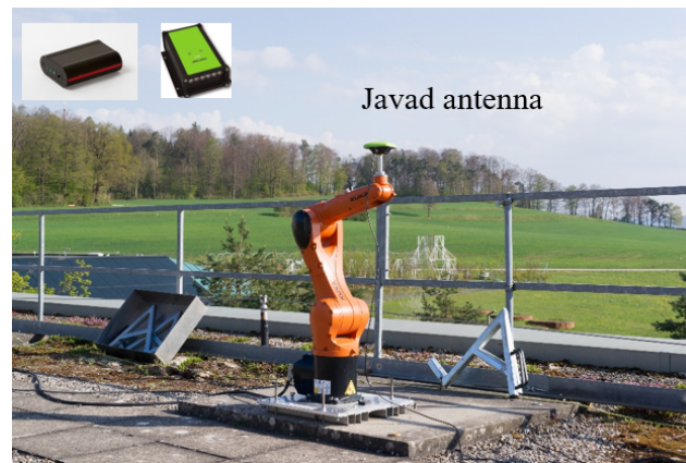
Figure 2. Experimental setup for the dynamic tests (session 1): a seismic strong-motion waveform was simulated using a KUKA robot arm. The same GNSS hardware was used as for the static kinematic test for station MON1.
