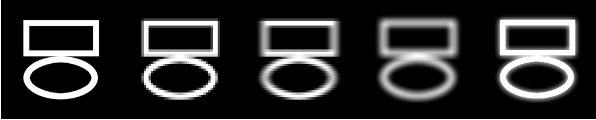
Figure 3.17: The passes to implement blooming . From left to right: The original image, the downsampled image, the horizontally blurred image, the complete blurred image, the final image.
