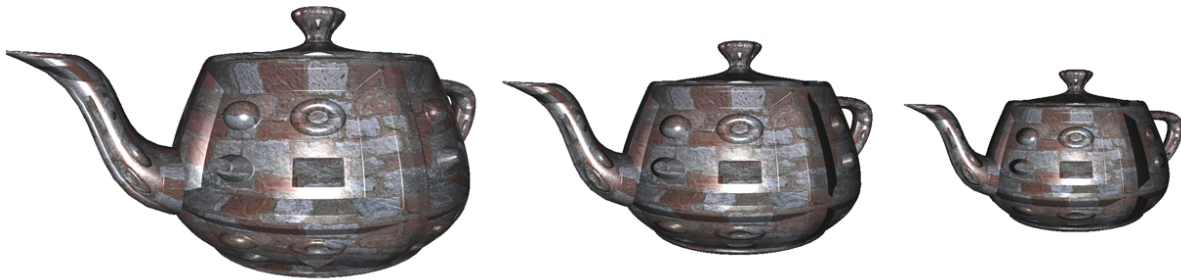
Figure 3.15: Example showing the effect LOD in use. From left to right: relief mapping , parallax mapping and normal mapping .
