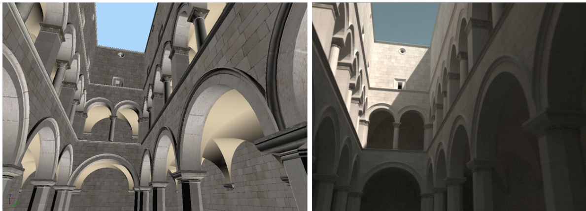
Figure 1.1: A comparison of a real-time rendered image ( \sim 500 frames per second) on the left and an image generated by a global illumination method on the right ( \sim 50000 seconds per frame). (Right image by Nick Chapman)
